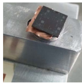
Fig 2. (Right) If samples are oddly shaped, too small, or too big for the pin-clip holder, then using adhesives is acceptable for these cases.
